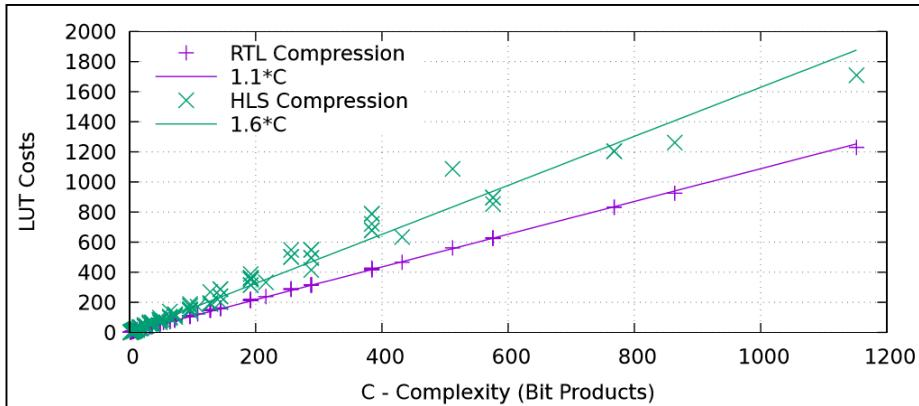
$C = \text{size of accumulator} * \text{size of weight} * \text{size of activation}$
