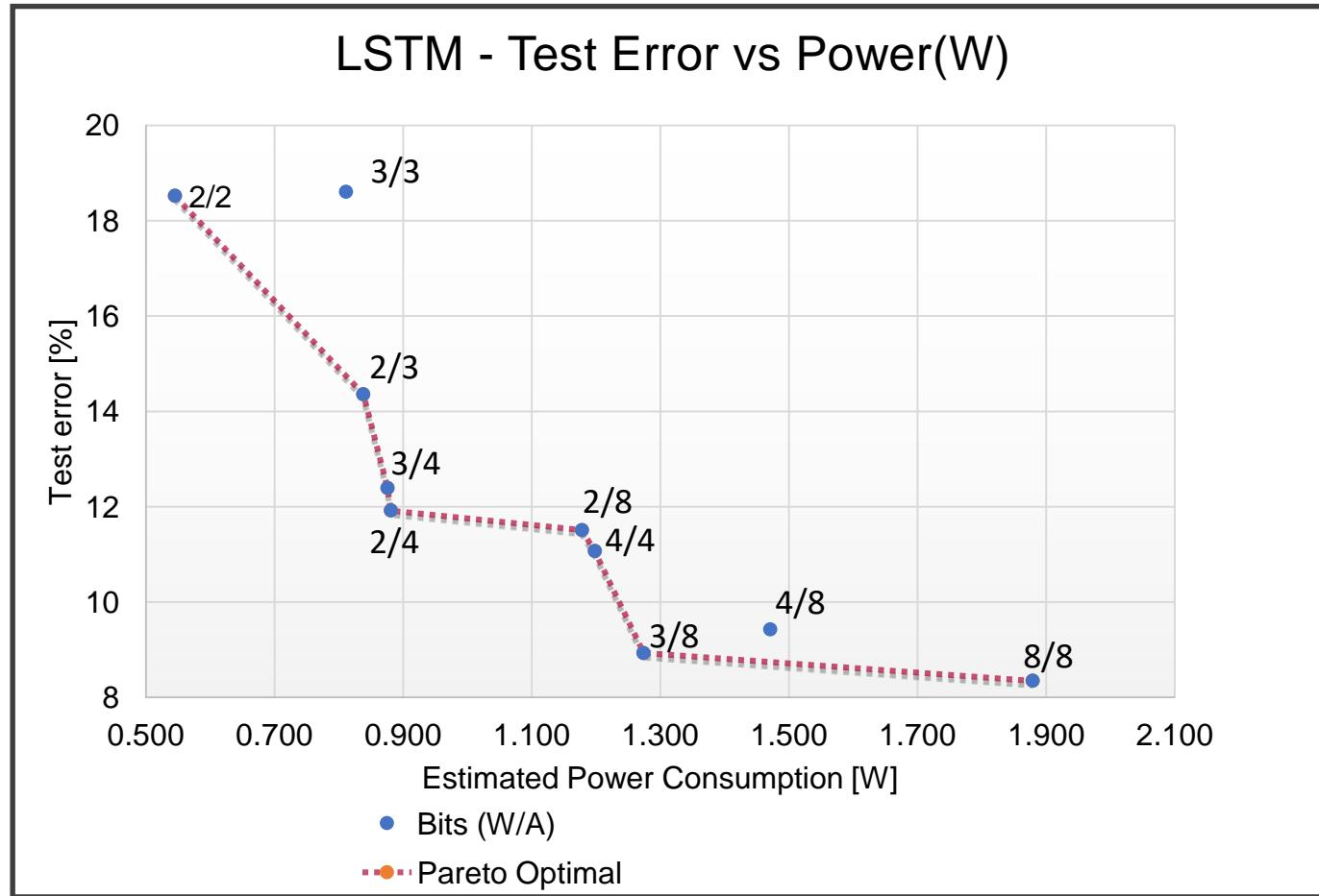
Target Device ZU7EV • Ambient temperature: 25 °C • 12.5% of toggle rate • 0.5 of Static Probability • Power reported for PL accelerated block only
