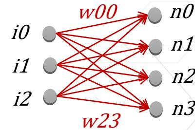
$$\begin{pmatrix} i0 & i1 & i2 \end{pmatrix} \times \begin{pmatrix} W00 & W01 & W02 & W03 \\ W10 & W11 & W12 & W13 \\ W20 & W21 & W22 & W23 \end{pmatrix} = \begin{pmatrix} n0' & n1' & n2' & n3' \end{pmatrix}$$
