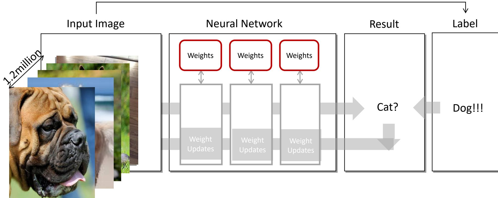
For ResNet50:       $1 \text{ epoch} \text{ takes } 1.2\text{M} * 23 \text{ Billion operations} = 23 * 10^{15} \text{ operations (peta)}$
